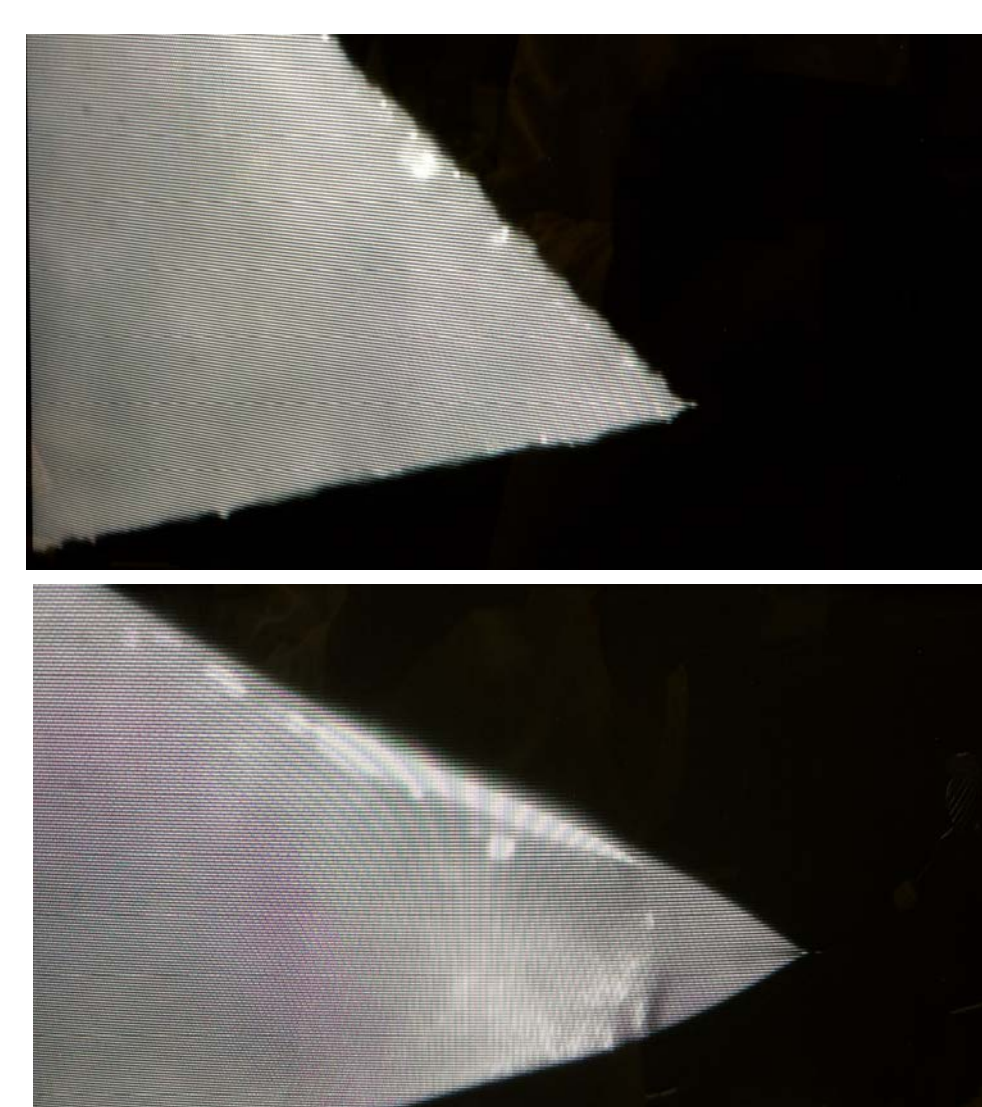
Figure 2. Top: Wetted paper tip, no HV applied. Viewed with camera mounted on MS
