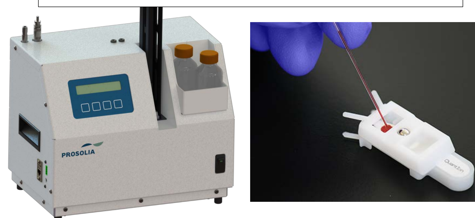
Figure 3. Picture of an automated paper spray MS attachment and the disposable paper spray cartridge
